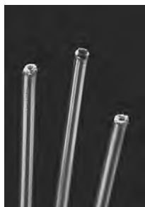
AVOID UNEVEN ENDS AND BURRS, DUE TO FILES (L) AND PLIER CUTS (R)
