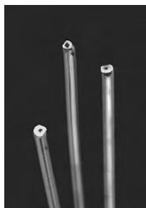
AVOID UNEVEN ENDS AND BURRS, DUE TO FILES (L) AND PLIER CUTS (R)
